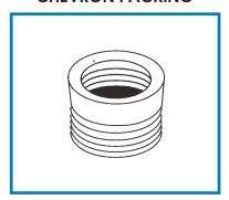
The ChemValve® Model 790EB-150 high performance lined plug valve has adjustable chevron TFM packing like a globe valve. The six ring set is much more substantial than the thin diaphragms used in other lined plug valve designs. If process pressure leaks into one of the packing rings, it will mechanically spread the ring sealing off the leak. This means there is little chance of either corrosive stem leakage onto the bonnet of the valve or fugitive emissions to the atmosphere.
